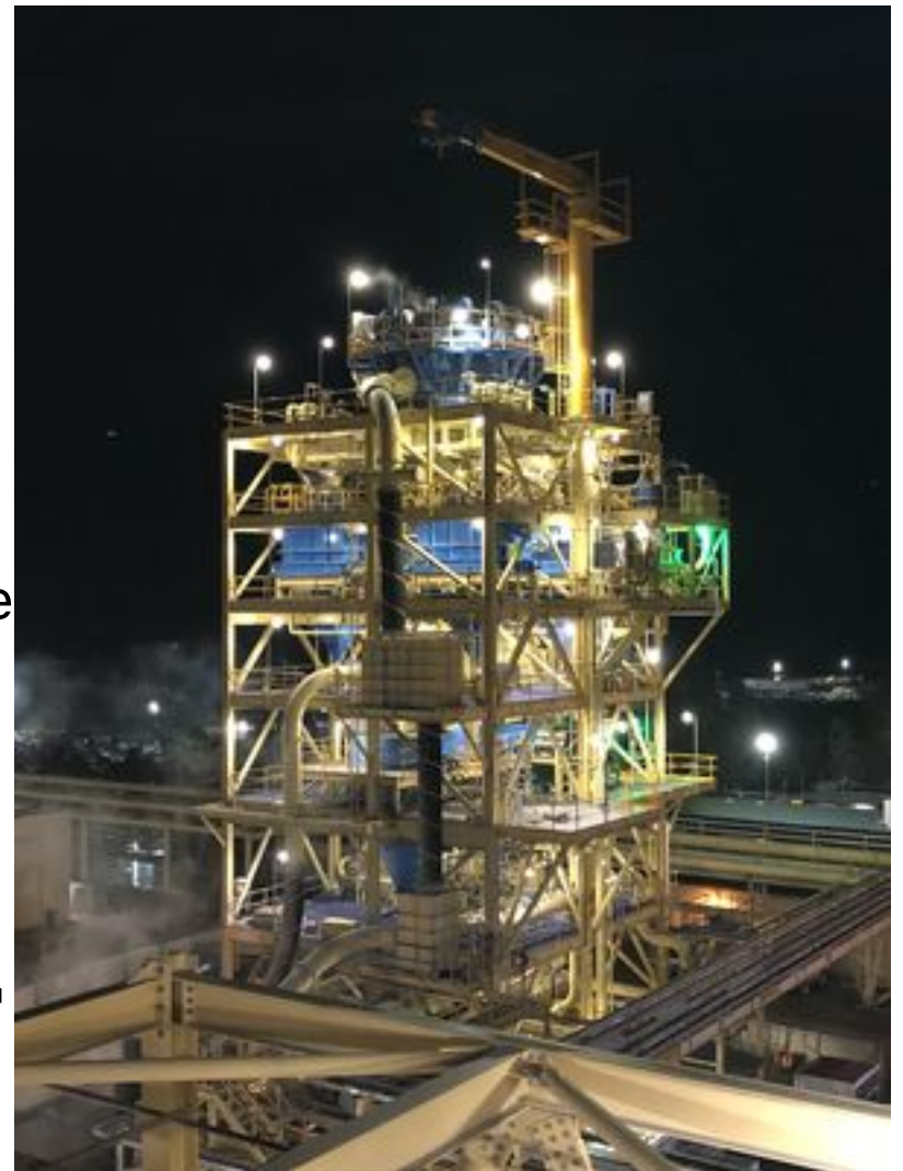
Newcrest Mining's Cadia facility in New South Wales, Australia, has already commercialised Eriez Flotation Division's HydroFloat for coarse flotation
