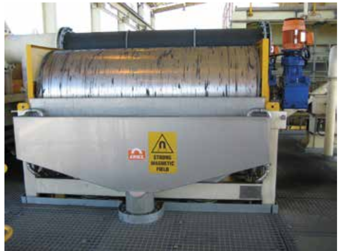
Model CDA Wet Drum Undergoing "In-Plant" Testing
