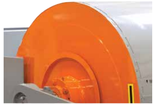
All Stainless Steel End Flange, Shell and Wear Wrap
