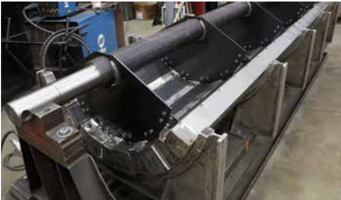
Construction of a wet drum magnet element
