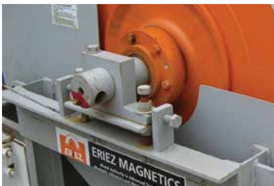
Self-Leveling Counter-Rotation Tank - Drum Positioning and Magnet Adjustment
