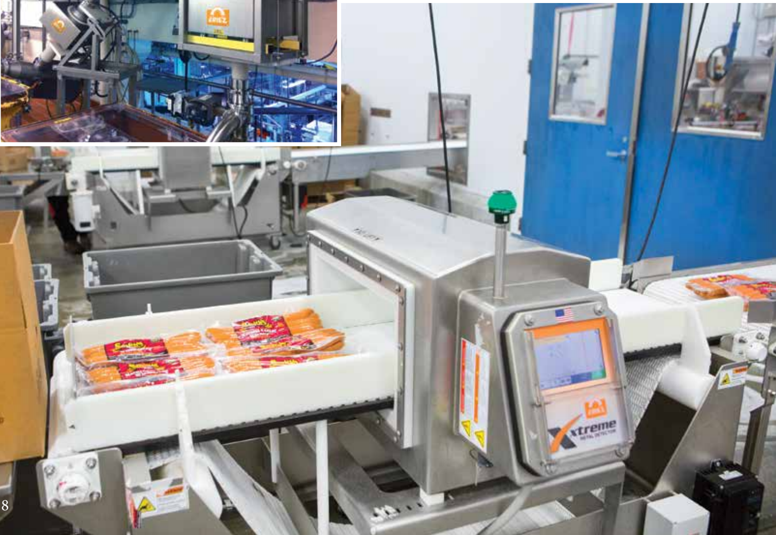
▼ Eriez' Xtreme® Metal Detector is installed in a hot dog packaging plant.
