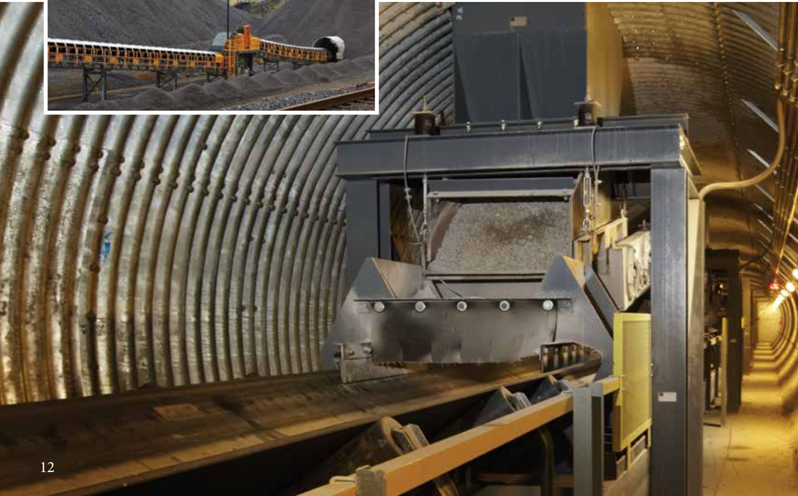
▼ Heavy duty mechanical feeders are found in high tonnage operations.
