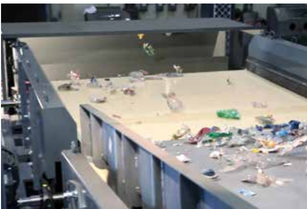
Eddy Current Separator sorts aluminum cans in a recycling facility.
